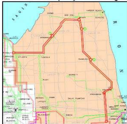
Figure 13 – Minimum 345 kV Transmission Requirements for Board-Identified Maximum Wind Capacity Level for Region 4
